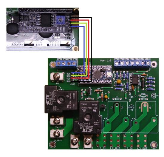
Connect mains, EV plug/socket, push button switch and current sensor (if used) to main board and power supply unit.
