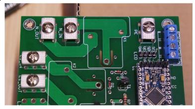
Solder relays to PCB. Please remember only 4 pin relays must be used with this PCB. Do not use 5 pin relays without modifying PCB!
