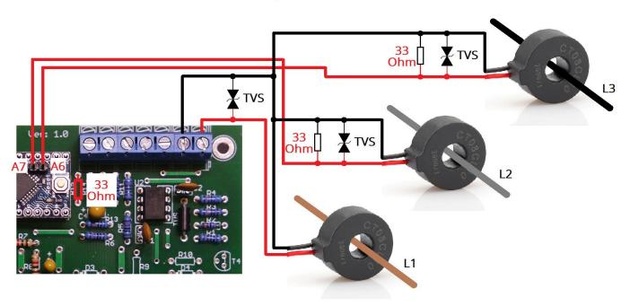
You might need to change current sensor calibration settings in EVSE settings menu, as SCT013-050 current transformer has inbuilt resistor of 290hm and EVSE code was written for SCT013-050 sensors. But this is not an issue as you can calibrate sensor readings by changing calibration settings. Please follow this link to see how to do this: <a href="https://youtu.be/XMWdDWNPO70">https://youtu.be/XMWdDWNPO70</a>.
