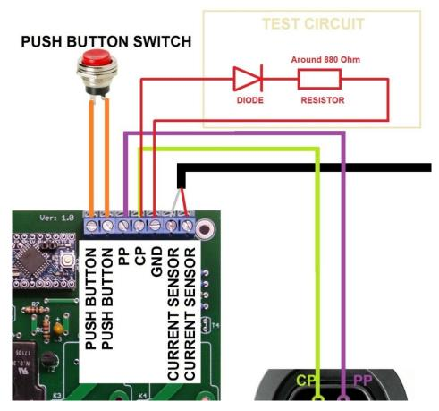
After you've connected test circuit, switch the mains power on again without touching any wires or components of your EVSE. This time you should hear relays clicking and LCD display showing "CHARGING" or battery symbol.
