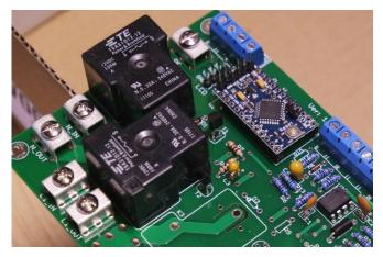
Please apply some solder on the bottom side of PCB on mains traces. This must be done to increase conduit size to make sure board will be able to withstand high currents.
