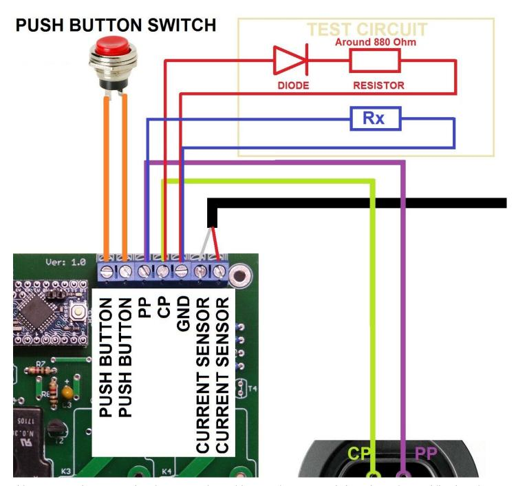
This test must be repeated 4 times, one time without resistor Rx, and then three times while changing resistor Rx. You should get following results while doing this test:
