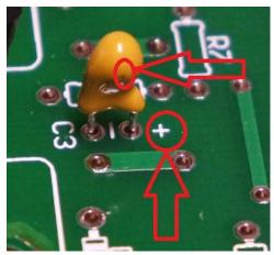
If you are using current sensor on your EVSE, then solder tantalum capacitor C4. Again keep attention on correct orientation.
