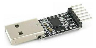
Please connect it with your Pro Mini as shown bellow. Please note that pins might be different on different converters and different Pro Mini boards, so always check pin markings.
