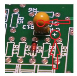
Solder LF353. Keep attention to correct component orientation.
