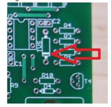
Solder transistors T1 and T2 (and T3, T4 for three-phase EVSE). Then fitting transistors please follow orientation marks on PCB.
