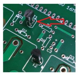
Solder diodes D1, D2, D5 (and D3, D4 for three-phase EVSE). Diode correct orientation also must be observed, please follow markings on PCB.
