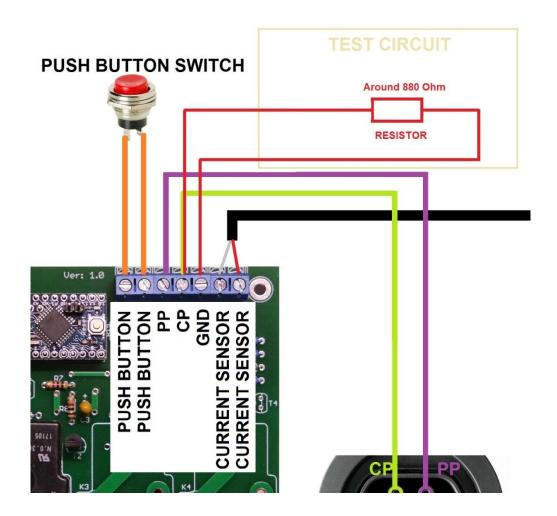
After you've connected test circuit, switch the mains power on again without touching any wires or components of your EVSE. This time you should see "EVSE CHK FAILED" on your EVSE LCD screen.
