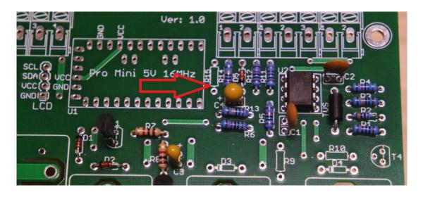
Solder pins for LCD connector X5.
