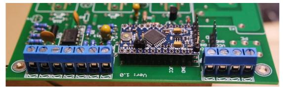
Solder screw terminals X6-X10 (X6-X14 for three-phase EVSE). Use high power soldering tool to make sure solder is done properly!
