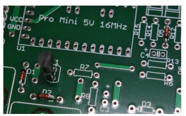
Solder ceramic capacitors C1 and C2. Orientation is not important on those.
