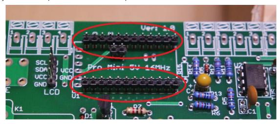
Solder the rest of pins to Pro Mini board facing upwards. These will be used for firmware updates and later developing. A6 and A7 will be connected directly to STC-013 current sensors on three-phase EVSE version.
