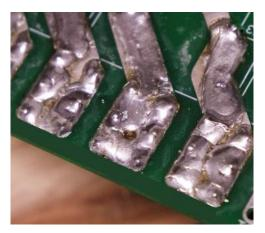
After soldering all components to PCB, it should look like in the picture below. Please note this picture shows single-phase non-tethered with current monitoring version of EVSE.
